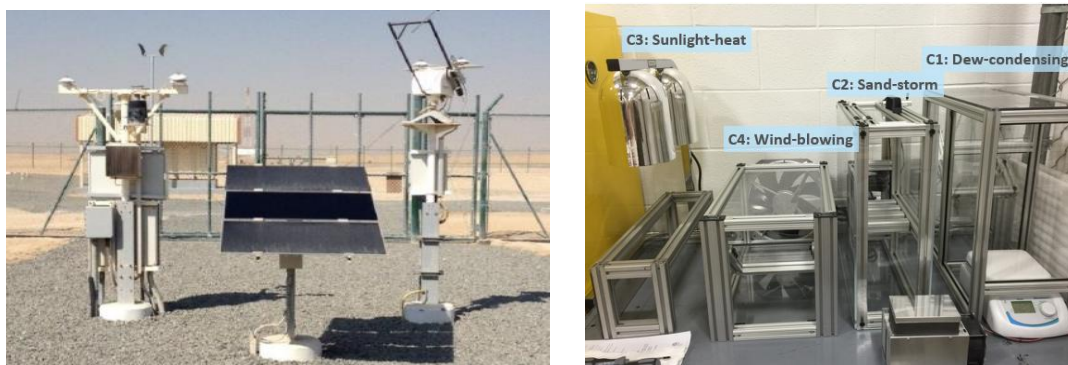
Figure 26 (left) Soiling monitoring station at test site in UAE. (right) Lab scale environmental simulator for anti-reflective coating development 59 .
