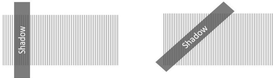
There is no risk of module damage due to “row-to-row” shading in landscape orientation. There is also no risk if shading occurs while modules are in open circuit conditions or no risk from diffuse shading for objects greater than 2 meters or 7 feet.
